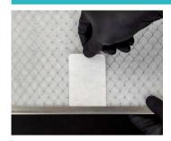
With fleece side facing up, tuck one end of **REPLACE**™ matrix under the prefilter frame. More than one **REPLACE**™ may be positioned on the prefilter if multiple samples or time-points for the health monitoring period are desired.
