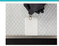
3 Secure the free end of REPLACE™ matrix with the supplied flat metal clip with the outer u-shaped portion of the clip on top of REPLACE™ and the inner tongue of the clip tucked under the prefilter wire mesh. The REPLACE™ and clip should be secure and flat against the prefilter.
