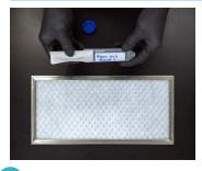
At the end of the monitoring period remove REPLACE™ from prefilter.
