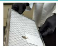
Place exhaust air prefilter onto rack with **REPLACE™** facing the oncoming cage exhaust airflow.
