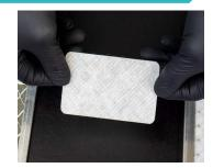
If the prefilter needs to be cleaned or replaced during the health monitoring period, remove **REPLACE™** and place on a clean surface or in a clean plastic bag. Reposition **REPLACE™** on new or cleaned prefilter as in steps 2-3 and place exhaust air prefilter onto rack as in step 4.
