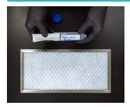
At the end of the monitoring period remove **REPLACE™** from prefilter. Curl REPLACE™ lengthwise with fleece-side-inward, place in labeled 50 mL conical tube and secure lid.
