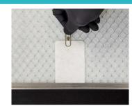
Secure the free end of **REPLACE™** matrix with the supplied flat metal clip with the outer u-shaped portion of the clip on top of **REPLACE™** and the inner tongue of the clip tucked under the prefilter wire mesh. The **REPLACE™** and clip should be secure and flat against the prefilter.
