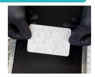
If the prefilter needs to be cleaned or replaced during the health monitoring period, remove REPLACE™ and place on a clean surface or in a clean plastic bag. Reposition REPLACE™ on new or cleaned prefilter as in steps 2-3 and place exhaust air prefilter onto rack as in step 4.
